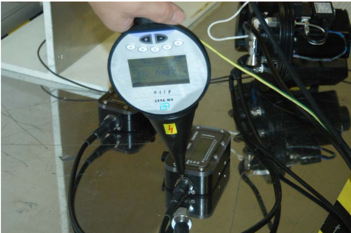
Photo 7 - System must recover normally after each static discharge
