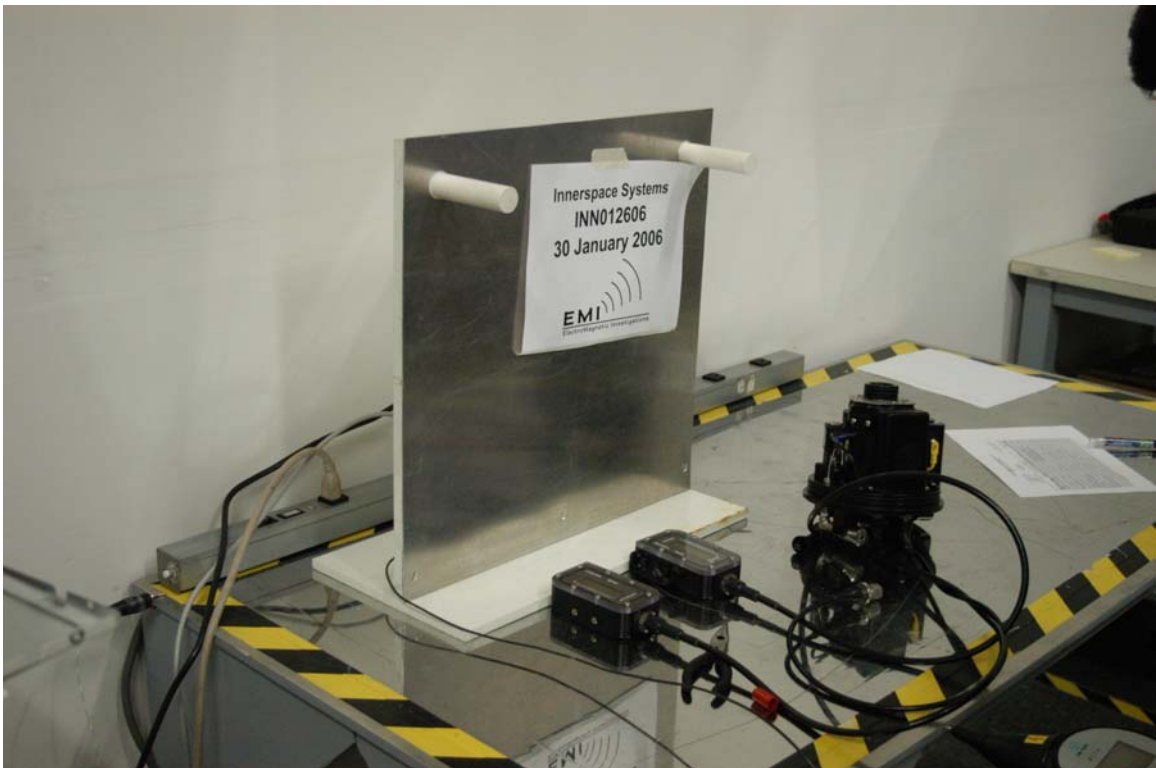
Photo 5 - Preparing APECS2 for ESD Static Discharge Testing
